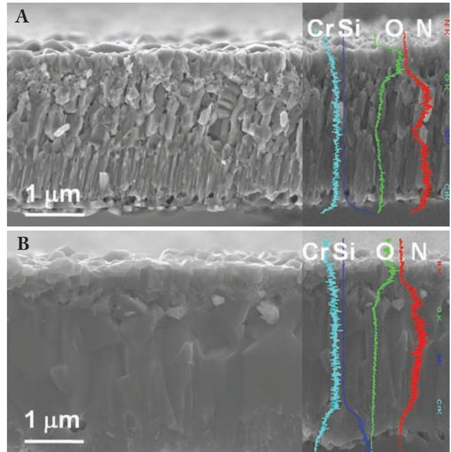
**Figure 8** – Cross-sectional SEM micrographs and corresponding Energy dispersive spectroscopy (EDS) line scans of the (A) DCMS and (B) MPP CrN coatings after annealing at 900  $^{\circ}\text{C}$  in an ambient air atmosphere.<sup>16</sup> (from reference 16 with permission, Elsevier)
