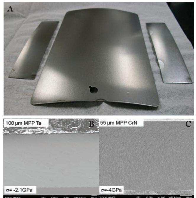
**Figure 6** – (A) a 20 μm CrN coating (10 μm/hr) deposited on 4x6 inch steel substrate; (B) cross-sectional SEM image of a 55 μm CrN coating (10 μm/hr)<sup>12</sup> (from reference 12 with permission, Elsevier); and (C) cross-sectional SEM image of a 100 μm Ta coating (16 μm/hr).<sup>14</sup> (from reference 14 with permission, IEEE)
