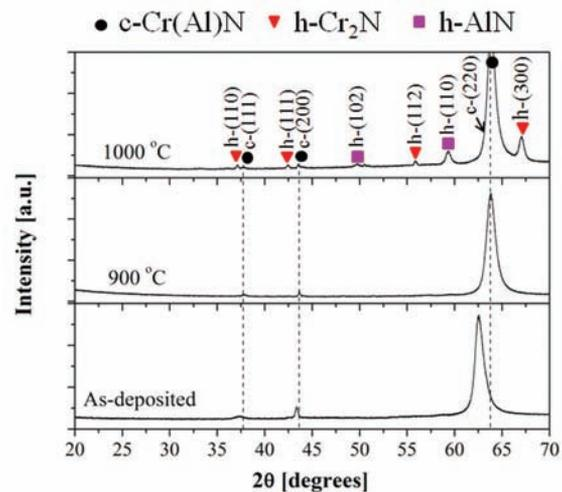
**Figure 9** – XRD patterns of the CrN-AlN coatings after annealing at 900–1000  $^{\circ}\text{C}$  showing no phase changes.<sup>13</sup> (from reference 13 with permission, Elsevier)
