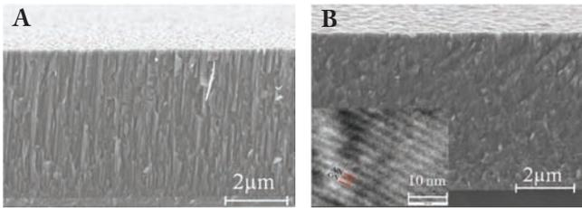
**Figure 4** – Cross-sectional SEM images of the CrN/AlN nanoscale multilayer films deposited by (A) dcMS and (B) MPP techniques. (The small insert TEM image shows that the modulation period of CrN/AlN nanolayers is 2.8 nm in this case)
