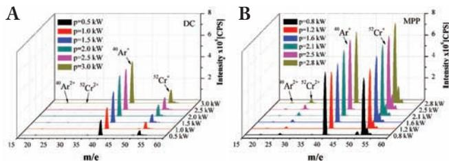
Figure 2 – Ion mass distributions for (A) dcMS and (B) MPP of Cr films.<sup>9</sup> (from reference 9 with permission, Elsevier)
