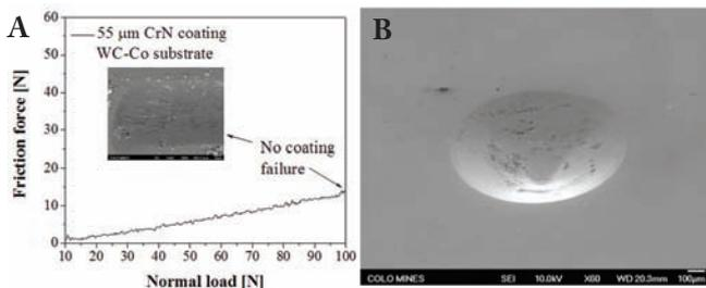
**Figure 7** – Friction force versus applied load during the progressive load scratch tests performed on (A) a 55  $\mu\text{m}$  CrN<sup>12</sup> (from reference 12 with permission, Elsevier) and (B) SEM image of the HRC indent on the thick MPP Ta coating after 150 kg load.<sup>14</sup> (from reference 14 with permission, IEEE)
