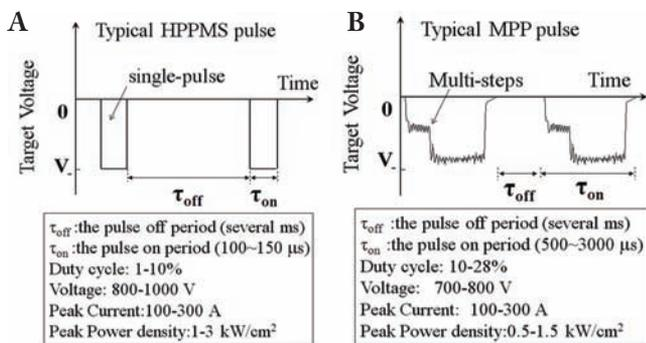
Figure 1 – Typical target voltage waveforms and parameters of (A) HPPMS and (B) MPP.<sup>8</sup> (from reference 8 with permission, AVS)
