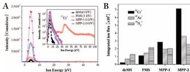
Figure 3 – (A) Comparison of the IEDs of Cr<sup>+</sup> and (B) Comparison of the integrated Cr<sup>+</sup>, Ar<sup>+</sup> and N<sup>+</sup> ion fluxes from the IED curves during reactive sputtering of CrN films under dcMS, PMS (100 kHz and 60% duty cycle) and two MPP conditions.<sup>11</sup> (from reference 11 with permission, Elsevier)
