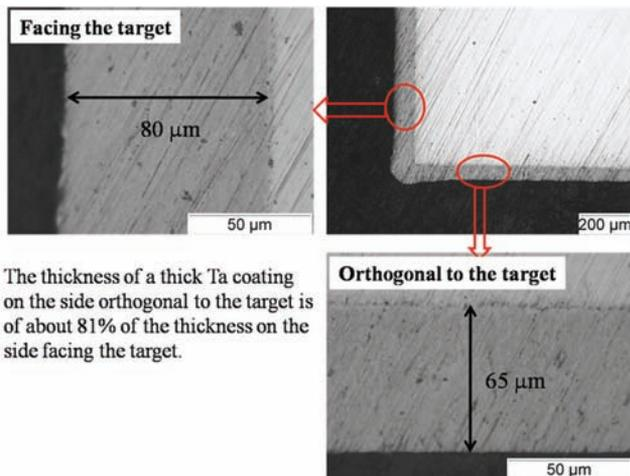
**Figure 5** – Optical images of an 80 μm thick α-Ta coating deposited using MPP showing a good homogeneity of the coating coverage on the side orthogonal to the target.<sup>14</sup> (from reference 14 with permission, IEEE)
